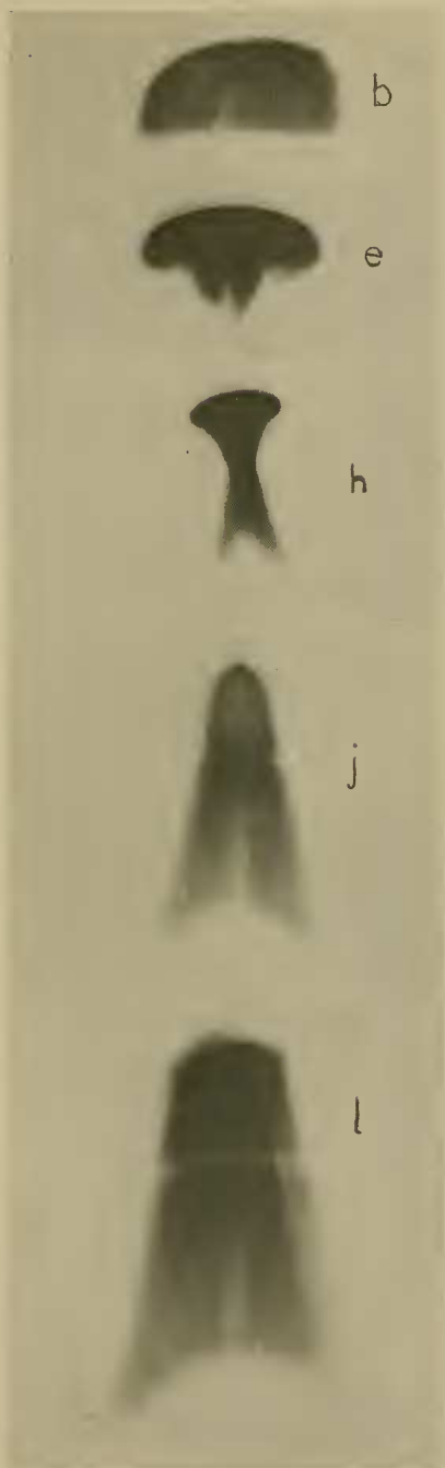
Fig. 2. Photographs showing the distribution of light at different planes in a beam of light passing through a focal region. The lettering is the same as in fig. 3.
